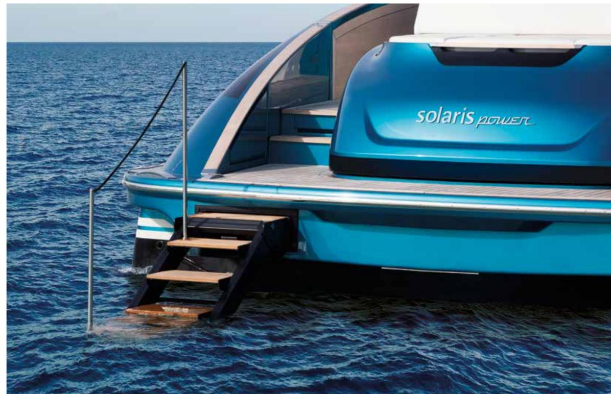
The hydraulic bathing stairs allow very comfortable to climb into the water, works as a gangway and is adjustable in height.
