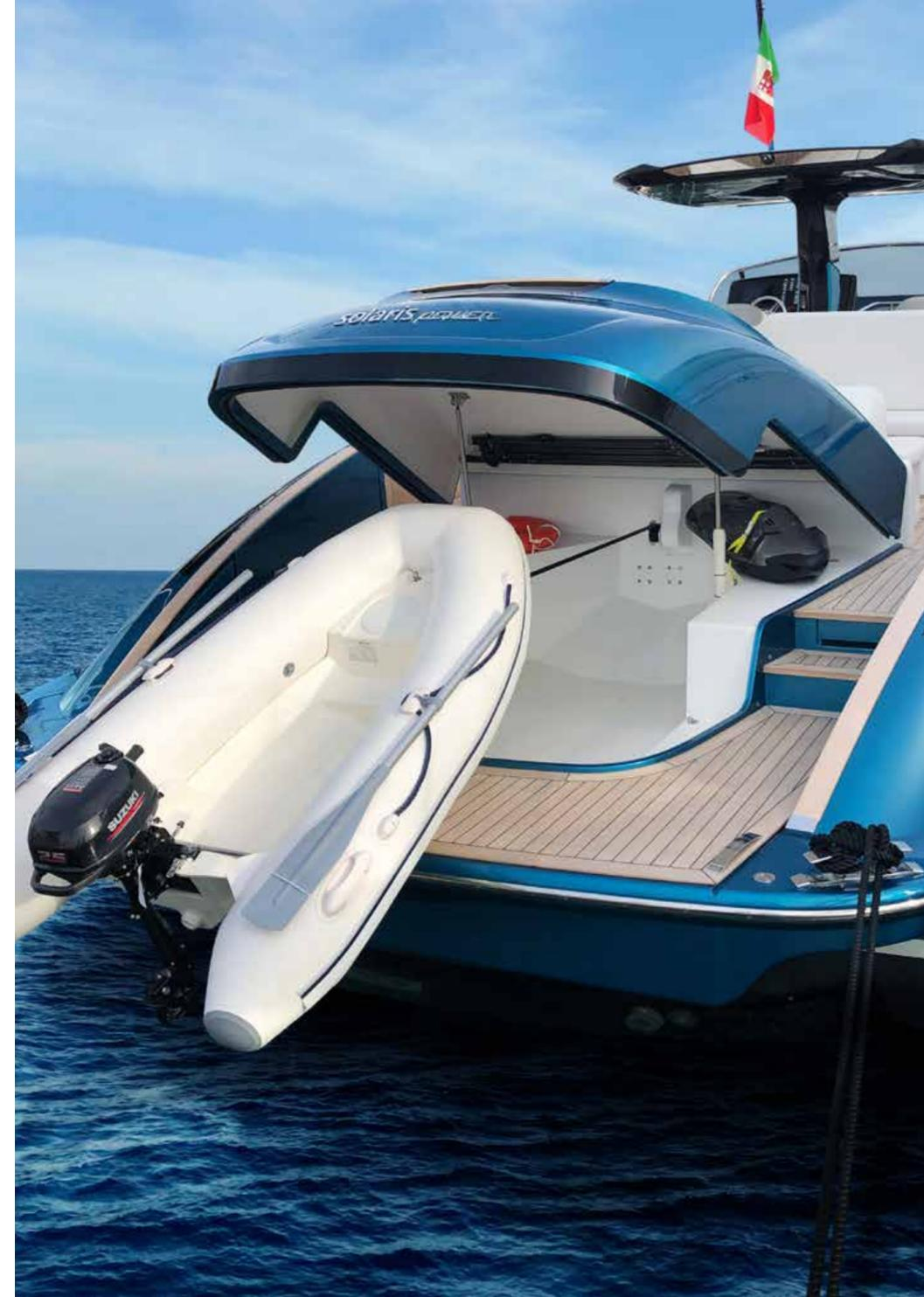
A single person by means of integrated winch and stainless steel sleds can carry out launching the tender easily. In the garage, there is also space for two Seabobs.
