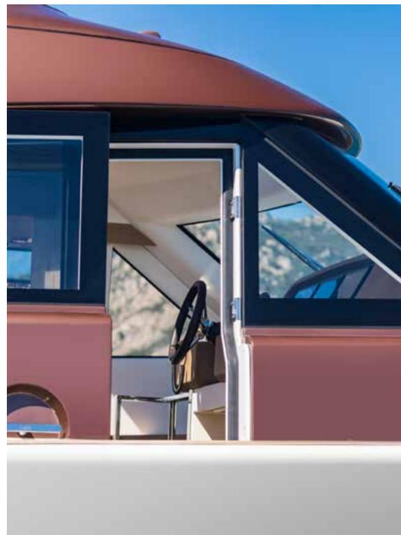
The side door at the helmsman brings great accessibility and flexibility, allows easy deck access without walking through the salon and is also an optimal ventilation for the salon.
