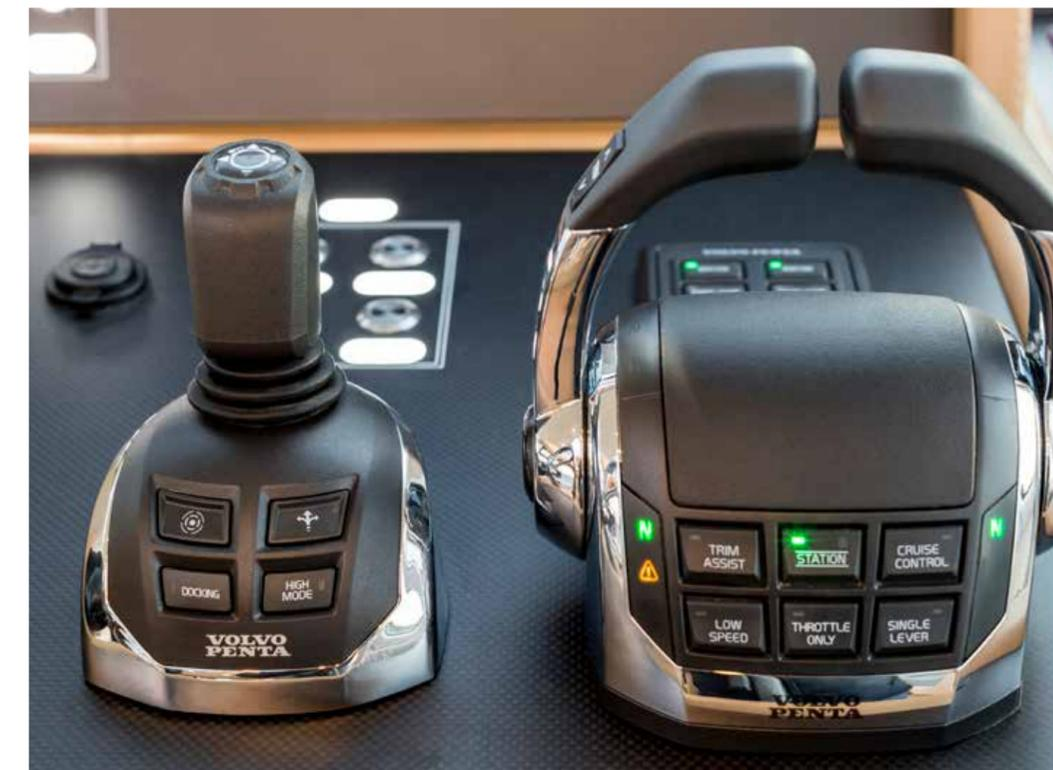
The joystick and the Azimutal iPod with differentiated simple control greatly facilitate port maneuvers and allows a single person to dock.
